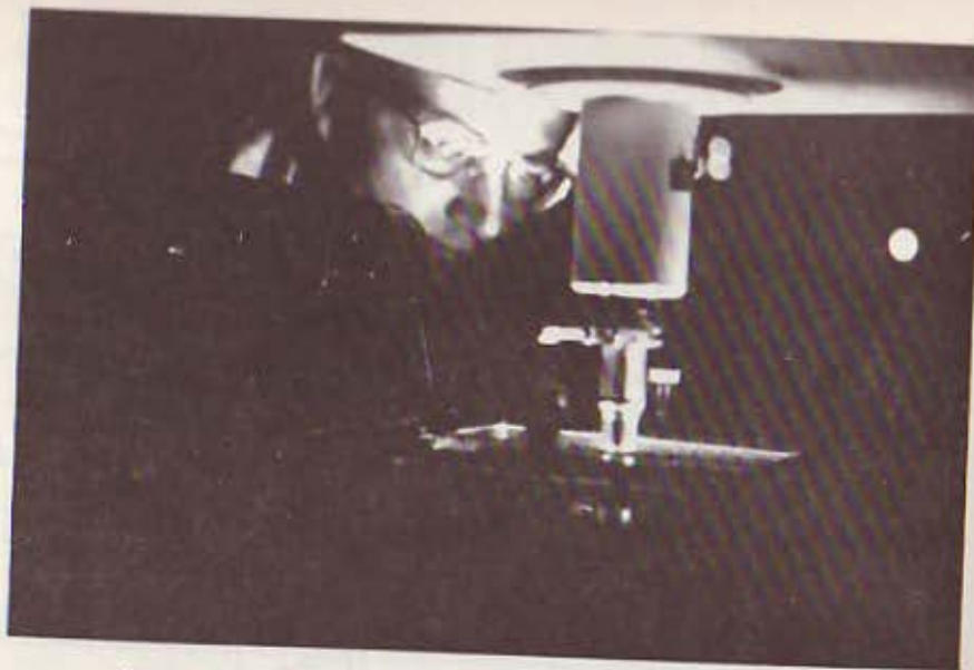
Figure 22. Lantern slide being scanned by microdensitometer.
